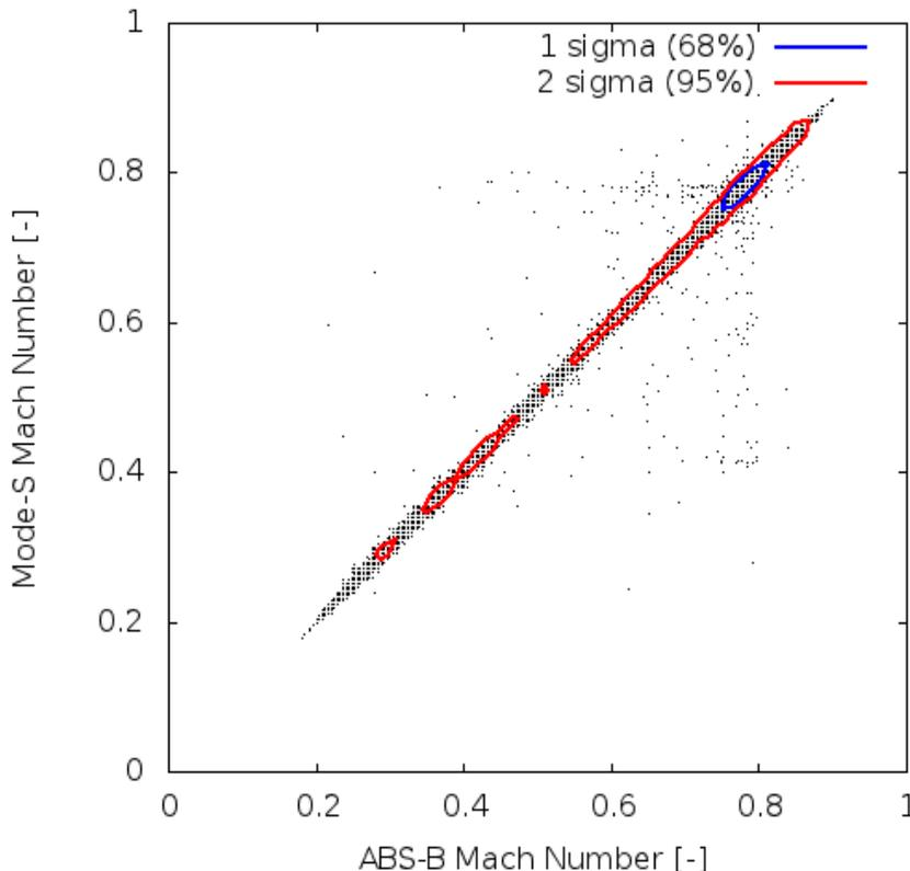
**Figure 13 : Comparison of Mach-number observations from ADS-B EHS and Mode-S EHS.**
