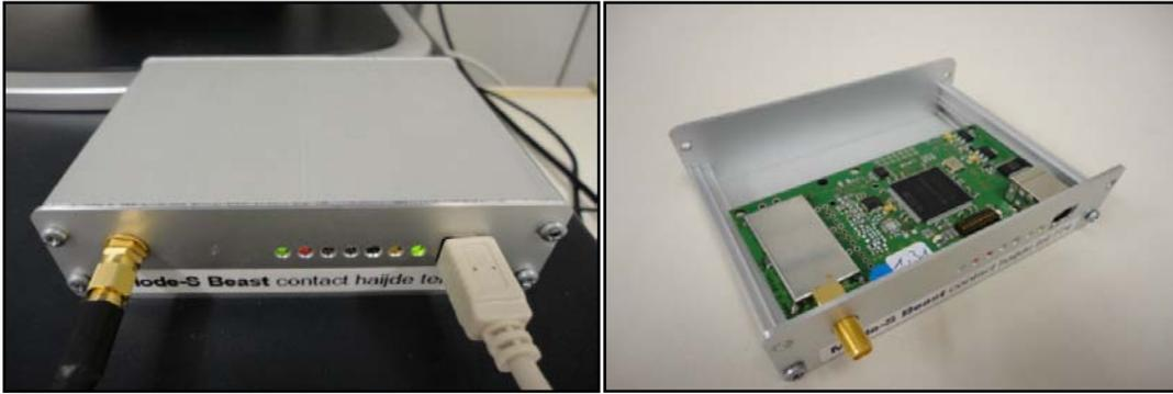
**Figure 2 :The Mode-S Beast "Series 2" in operation (left) and the PCB inside the housing (right).**
