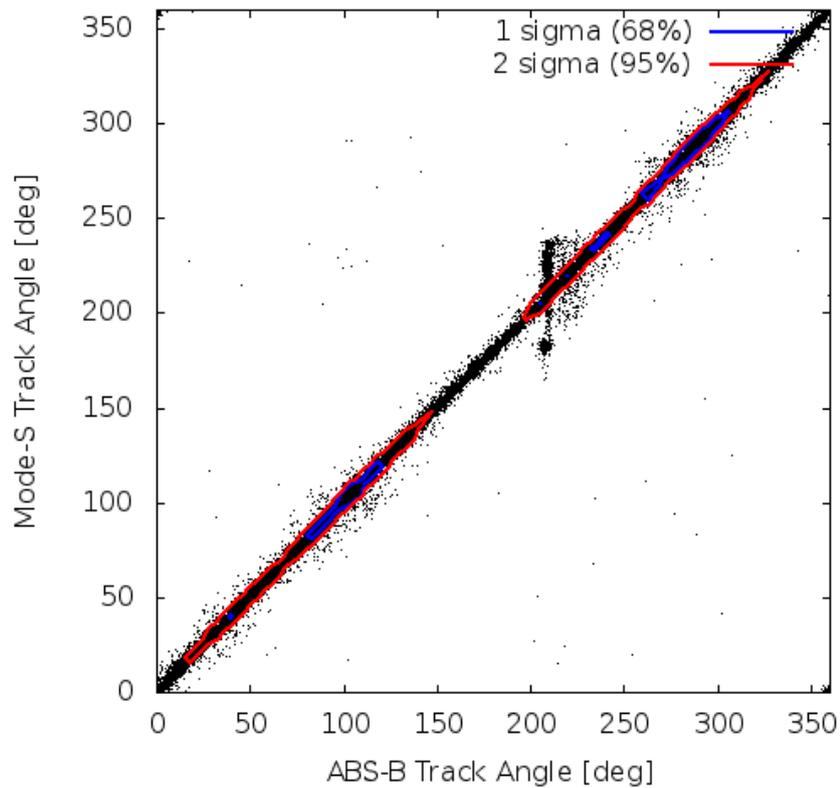
**Figure 18 : Comparison of track angle observations from ADS-B EHS and Mode-S EHS.**
