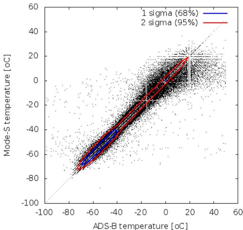
**Figure 19 : Comparison of Mode-S EHS and ADS-B EHS temperature observations.**
