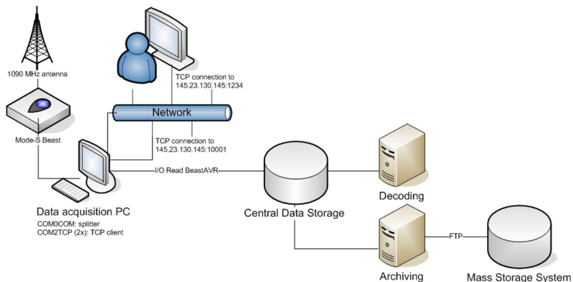
Figure 1 : Schematic overview of the Mode-S Beast data acquisition chain.
