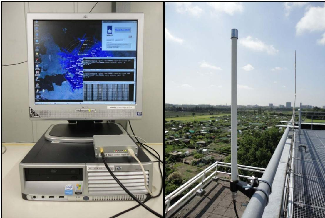
Figure 5 : Data acquisition PC and Mode-S Beast (left) and GP1090 antenna on the roof of the KNMI premises (right).
