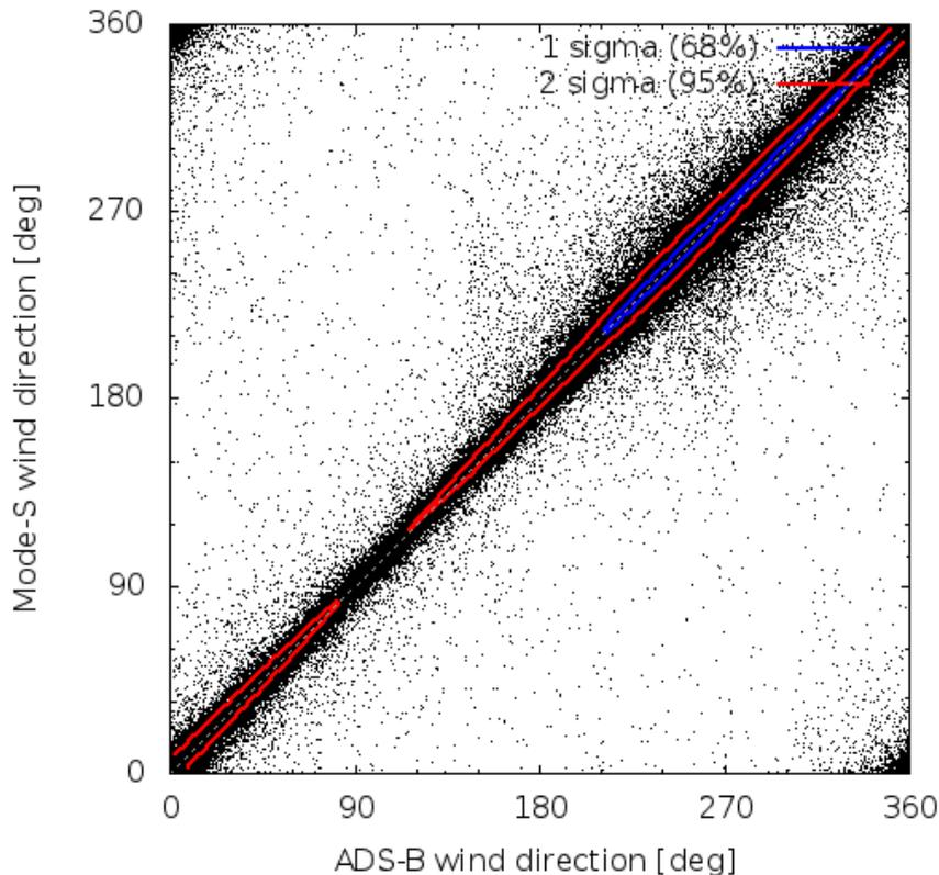
**Figure 21: Comparison of Mode-S EHS and ADS-B EHS wind direction observations.**
