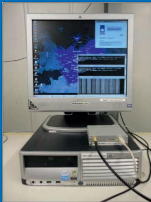
Figure 6: Data acquisition PC and Mode-S Beast (left) and GP1090 antenna on the roof of the KNMI premises (right).
