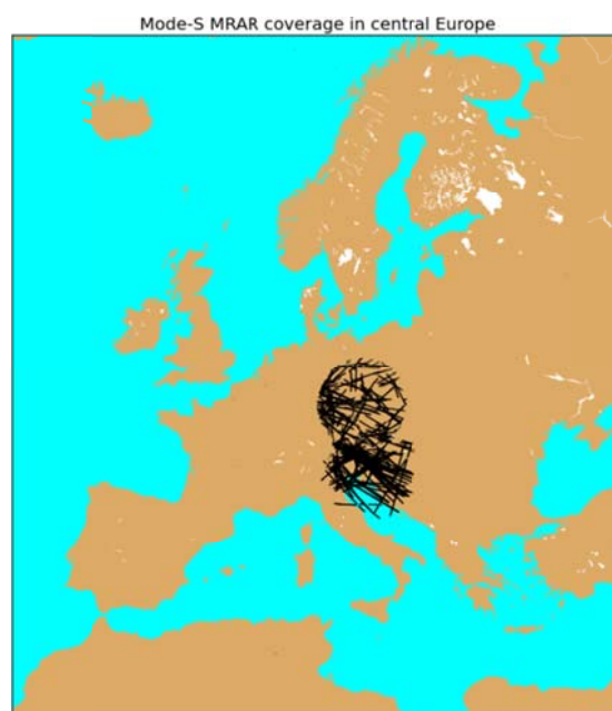
Figure 21: Area currently covered by MRAR data from 6 Mode-S radars in central Europe (Kastrup data is not shown).
