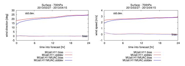
Figure 3: Impact on wind direction and wind speed. Comparison of Mode-S EHS MUAC observations between surface to 700hPa with independent forecasts ranging from +00 (analysis) to +24.
