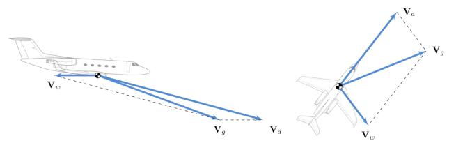
Figure 2: Geometry of an aircraft's path with respect to air and ground.
