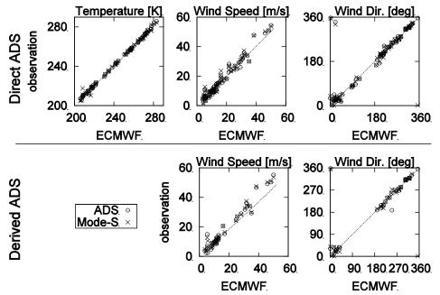
**Figure 2:** Scatter plots showing ECMWF temperature and wind versus ADS-C (direct and derived) and Mode-S.
