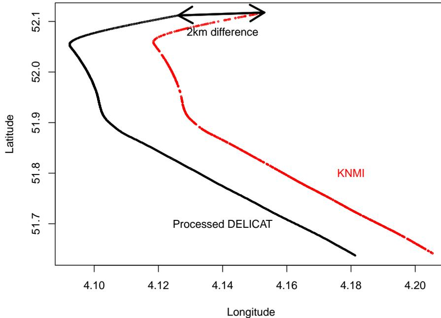
**Figure 4.** Comparison of flight paths as recorded by the KNMI receiver (red dots) and resulting from the processing of the DELICAT data (black dots) for a fragment of FL9. The 2 km error can be attributed to IRS drift which is of the order of 3 km per hour. IRS was calibrated prior to each flight.
