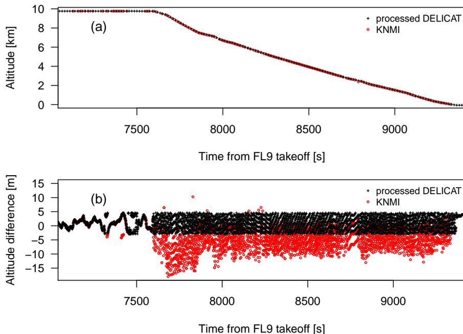
**Figure 3.** A comparison between the processed DELICAT data (black crosses) and KNMI data (red circles) of **(a)** the altitude profile (note that for the sake of clearness 97 % of the observations are not plotted here) and **(b)** the difference of the altitude with respect to the DELICAT reference altitude.
