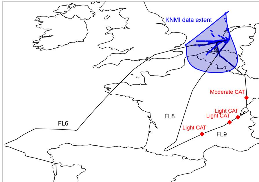
**Figure 1.** Tracks of DELICAT flights FL6, FL8 and FL9 (black solid lines). Peak turbulent events (red markers and red caption). KNMI data (blue dots) and KNMI data range (light blue shape).
