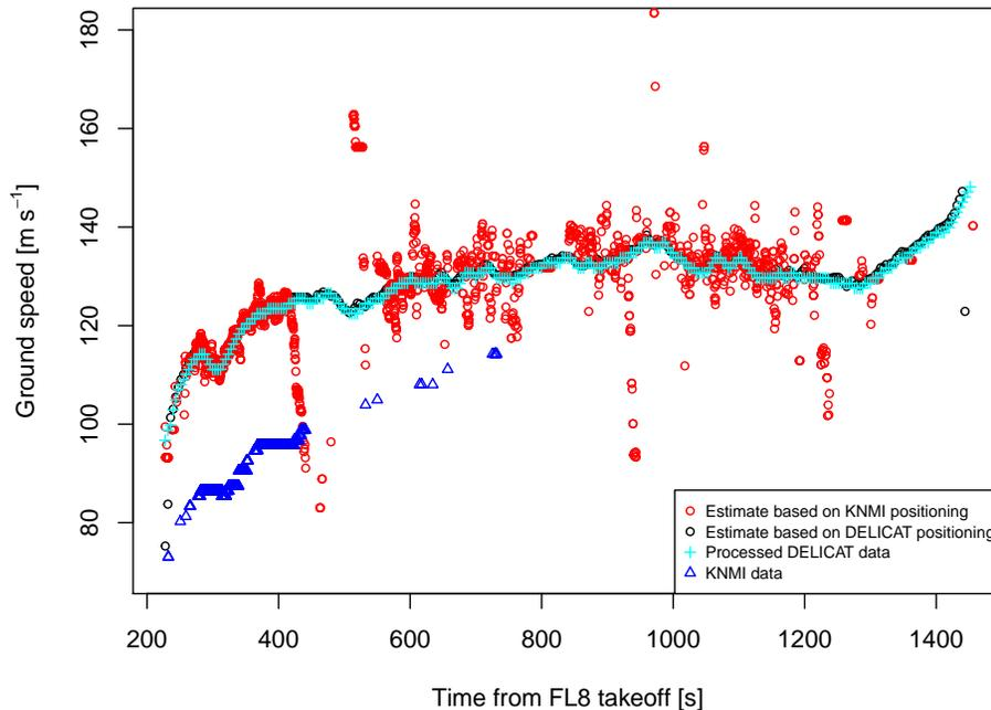
**Figure 5.** Comparison of ground speed record against estimates based on reported geographic position for the case of FL8. FL8 is presented because of the longest continuous KNMI record containing ground speed.
