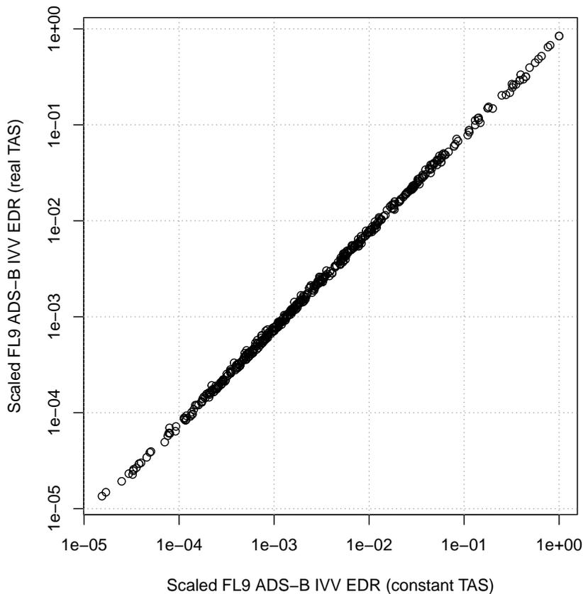
**Figure 10.** An exemplary comparison of EDR for FL9 calculated using IVV method using the real TAS record vs. the constant TAS approximation. We used  $250 \text{ m s}^{-1}$  as the constant TAS. Both of the EDR estimates were scaled to the range of values of constant TAS EDR thus are unitless and in approximate range 0–1.
