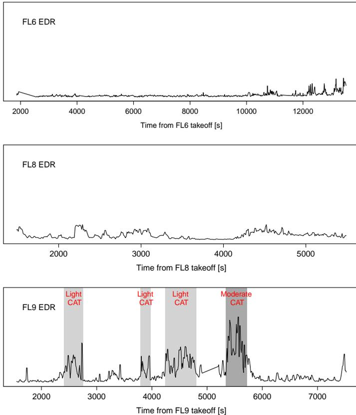
**Figure 2.** Reference EDR recordings from the DELICAT flights FL6, FL8 and FL9. Plots show 15s maxima of the EDR in the cruise fragments of the flights. Vertical scale is arbitrary (yet the same on all plots) as EDR is scalable by a constant. Shaded areas in FL9 pane are the CAT occurrences (as in Fig. 1).
