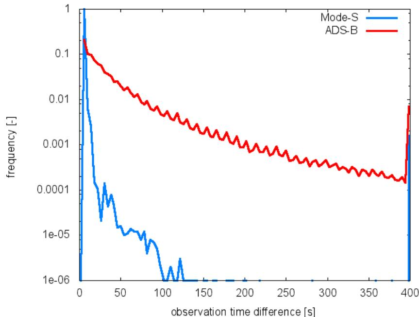
**Figure 12: Frequency distribution of the time difference of subsequent wind observations from Mode-S EHS (blue) and ADS-B EHS (red).**
