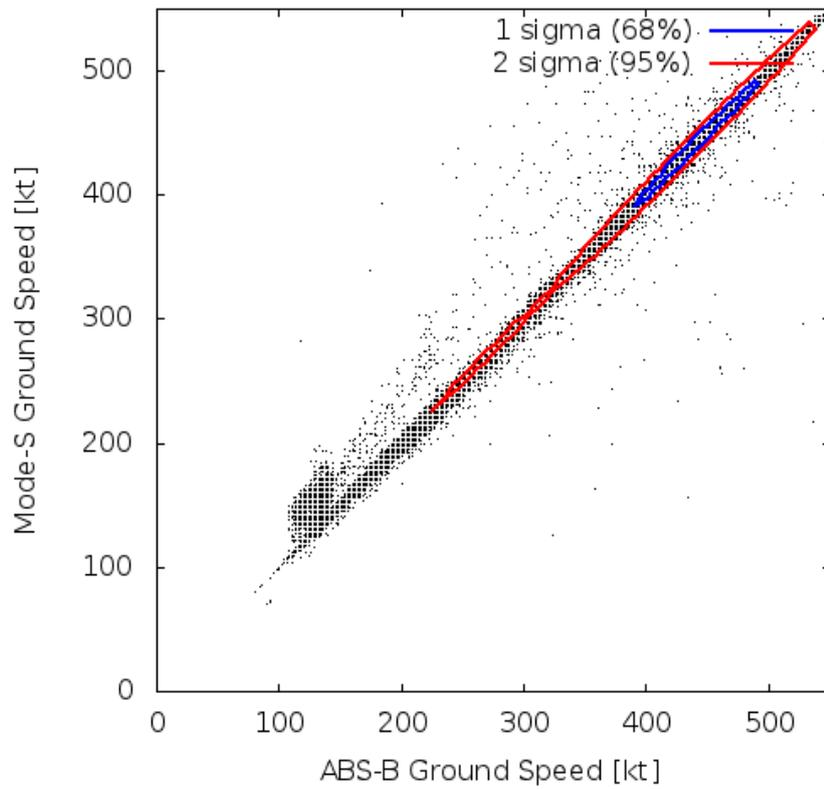
Figure 17 : Comparison of ground speed observations from ADS-B EHS and Mode-S EHS.
