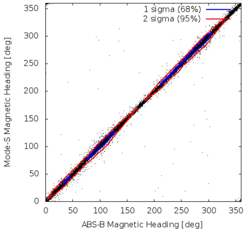
**Figure 16 : Comparison of magnetic heading observations from ADS-B EHS and Mode-S EHS.**
