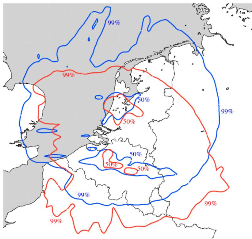
**Figure 10 : Relative horizontal coverage of the total number of Mode-S EHS wind and temperature observations retrieved from ATC (blue) and ADS-B EHS (red) data during nine days (1-9 April 2012).**
