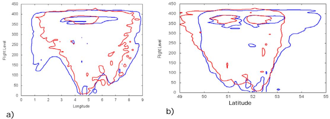
**Figure 11: a) Vertical coverage along the longitude of Mode-S EHS from ATC (blue) and ADS-B EHS from KNMI receiver (red); b) Vertical coverage along the latitude.**
