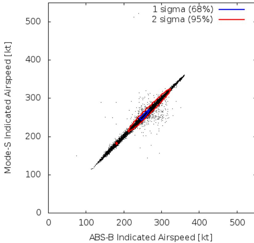
**Figure 15 : Comparison of indicated airspeed observations from ADS-B EHS and Mode-S EHS.**
