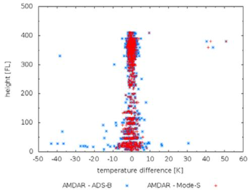
**Figure 22: Temperature difference of AMDAR and Mode-S EHS (red crosses) and ADS-B EHS (blue stars), respectively versus height.**
